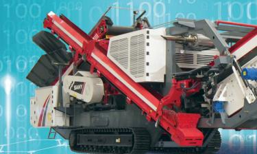
It is used for secondary and tertiary crushing and recycling of hard materials with compressive strength not exceeding 300Mpa in construction, transportation, railway, cement, building materials, metallurgy, tailings and other industries.
